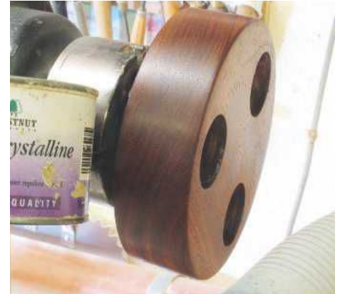
▲ Pic.15 Les is using microcrystalline wax, a modern wax finish with a higher melting point than traditional paste waxes so it will withstand more handling without dulling
